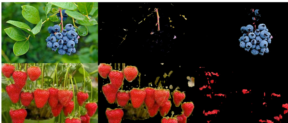
Figure 6: Left original RGB images, Centre modified NDVI output for detecting ripe fruit and right the implementation of modified NDVI (original image - sky -veg = fruit). This shows the worst and best of both methods.
